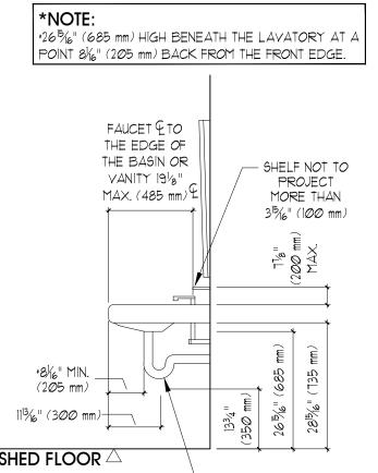
FINISHED FLOOR HAVE INSULATED PIPES OR WATER — SUPPLY TEMPERATURE LIMITED TO A MAX. OF 43°C TO PREVENT BURNS
